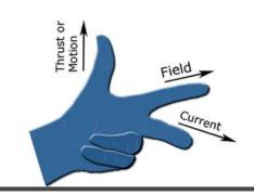
A force acts on a current-carrying conductor in a magnetic field. Fleming's left-hand rule shows the relative
